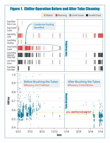
fouling and scaling had become a problem. After the condensor cleaning in December 2013, the warnings ended and chiller efficiency improved by 6 percent. SMARTenergy OPS<sup>®</sup> provides you with the data on performance and cost impact that can be needed to justify maintenance expenditures.
