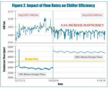
Continuous commissioning of the chilled water system from 2013 to August 2016 using SMARTenergy OPS<sup>®</sup> saved 1,600,000 kWh and \$111,000, yielding a 1.2 year payback.
