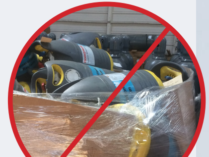
Shipping box not intact, cylinders not stacked
